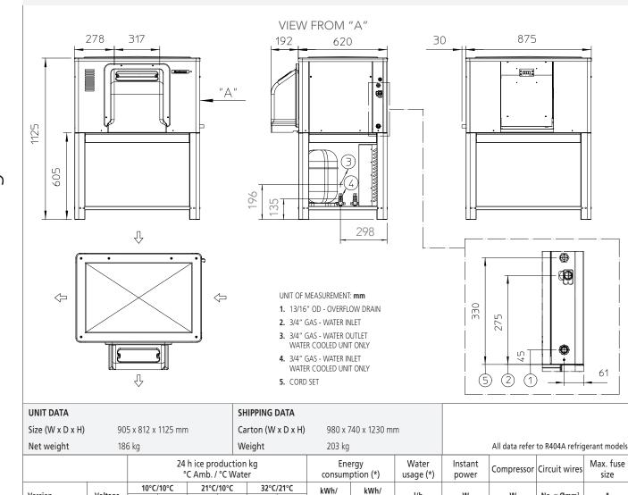
No. x Ømm<sup>2</sup> Version Voltage l/h w W 1 mm 2 mm 1 mm 2 mm 1 mm 2 mm 100 kg 24h MAR 76 AS 400/50/3N 2500 2250 5 x 1.5 570 510 0 460 0 395 15.0 60.0 16.5 MAR 76 WS 400/50/3N 330.0 570 510 0 0 0 0 15.0 60.0 2500 2250 5 x 1.5 MAR 76 AS 230/60/3 4 x 1.5 0 0 0 0 0 0 15.0 60.0 16.7 5000 2250 MAR 76 AS 380/60/3N 0 0 0 0 0 0 15.0 60.0 16.7 2500 2250 5 x 1.5 (Te -23.3°C; Tc +54.5°C) Compressor:
